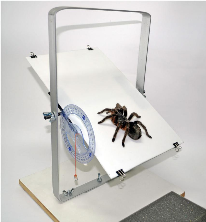
**Fig. 5. Experimental apparatus with a rotatory platform and a goniometer to measure the angles. Surfaces of the platform can be changed.**
